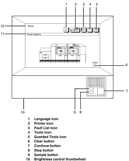
Figure 3-2. Printer control console
